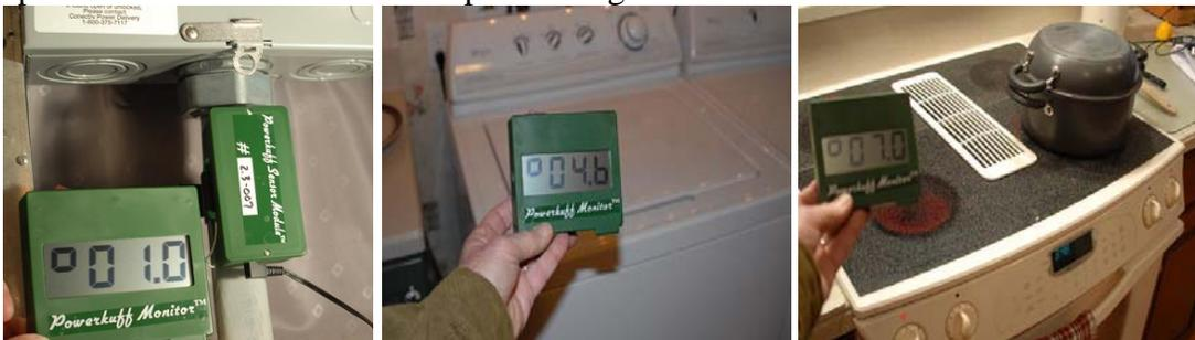
Take the display inside and demonstrate that the Powerkuff monitor is reading the power coming into your home by turning on or off a light or appliance and watch the power use numbers change. (Wireless range 30 meters or 100 feet)
