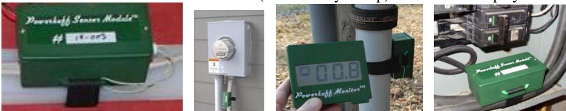
The Powerkuff monitor measures total electric power traveling in the service entrance cable which feeds the home or business. If you see 000.8 on the monitor your home is using 0.8 kilowatts or 800 watts of power right then. Powerkuff Monitor is like a speedometer to measure electric power usage.
